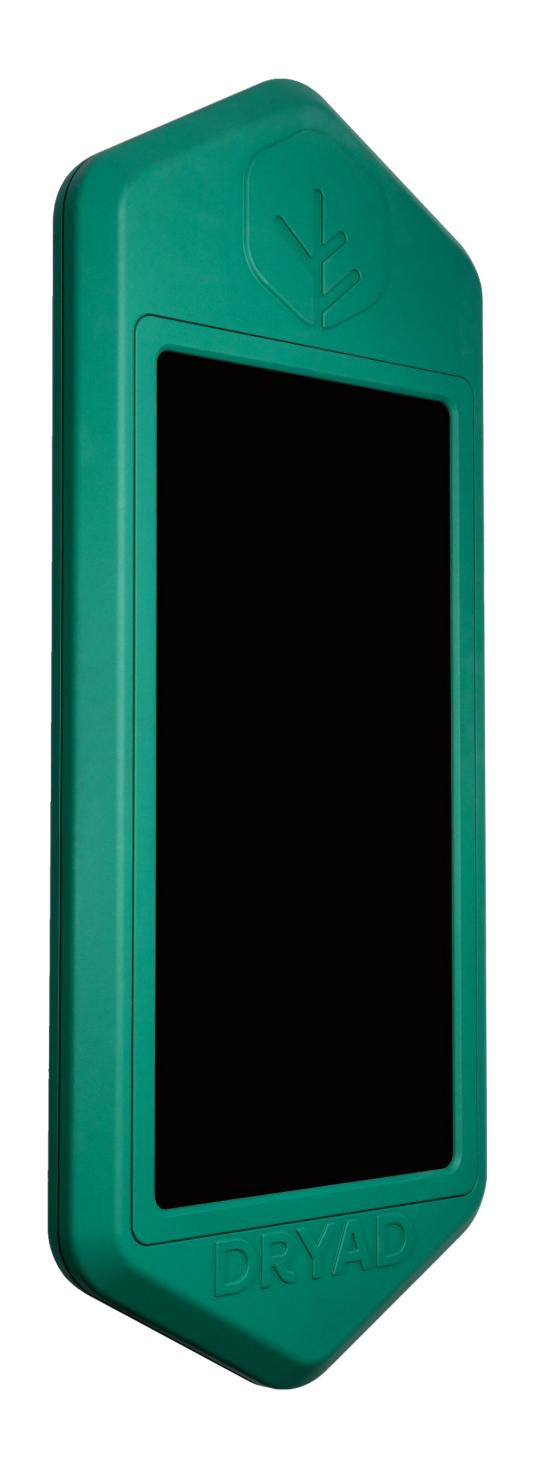
The Silvanet Mesh Gateway expands the Silvanet Network for large-scale deployments using a patent-pending multi-hop LoRaWAN mesh network, far beyond the range of standard single-hop gateways.
